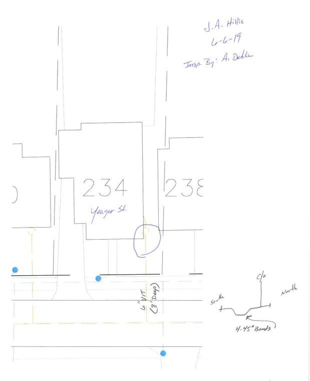
Justalled New Cleanort and replaced Broken VIT trap.
